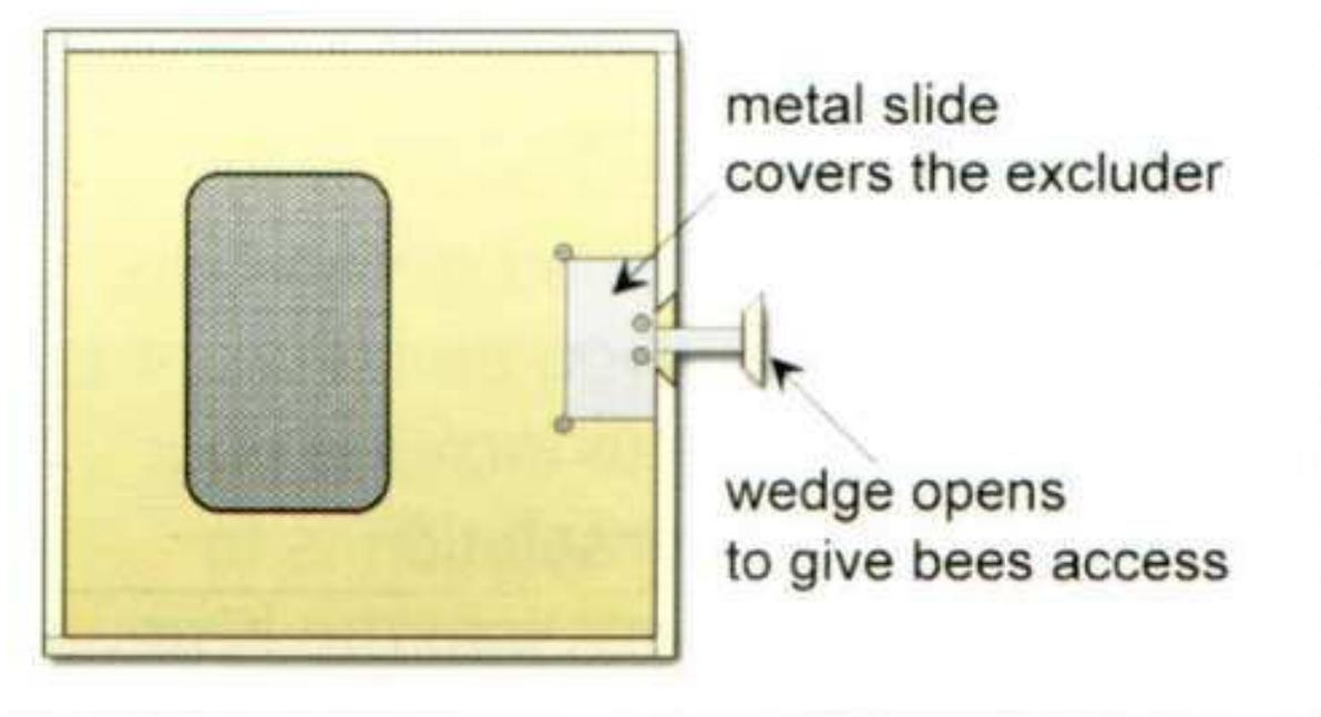
The Horsley board with the wedge open giving the bees access and closing the queen excluder to prevent movement between the two boxes
